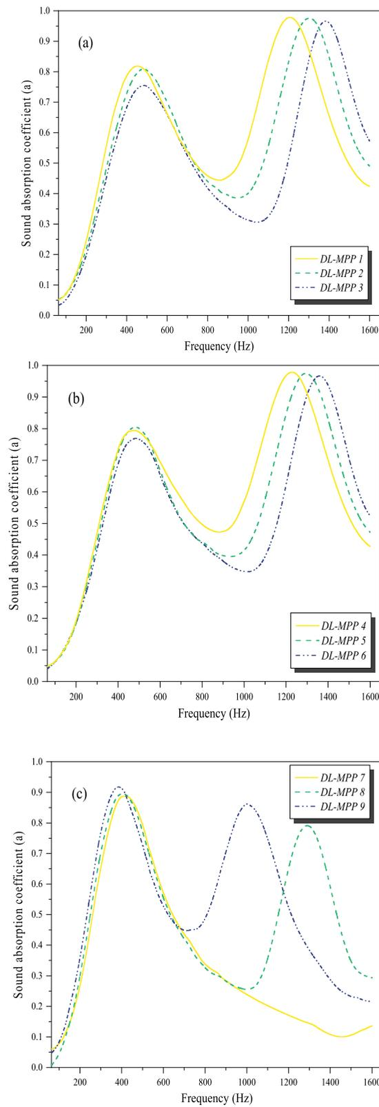
**Fig. 16.** The impacts of modifying the parameters of the second layer on the values of the acoustic absorption coefficient of DL-MPP sound absorbers a) increasing the diameters of the perforations (d), b) decreasing the thickness (t), c) the distance between the perforations (b).
