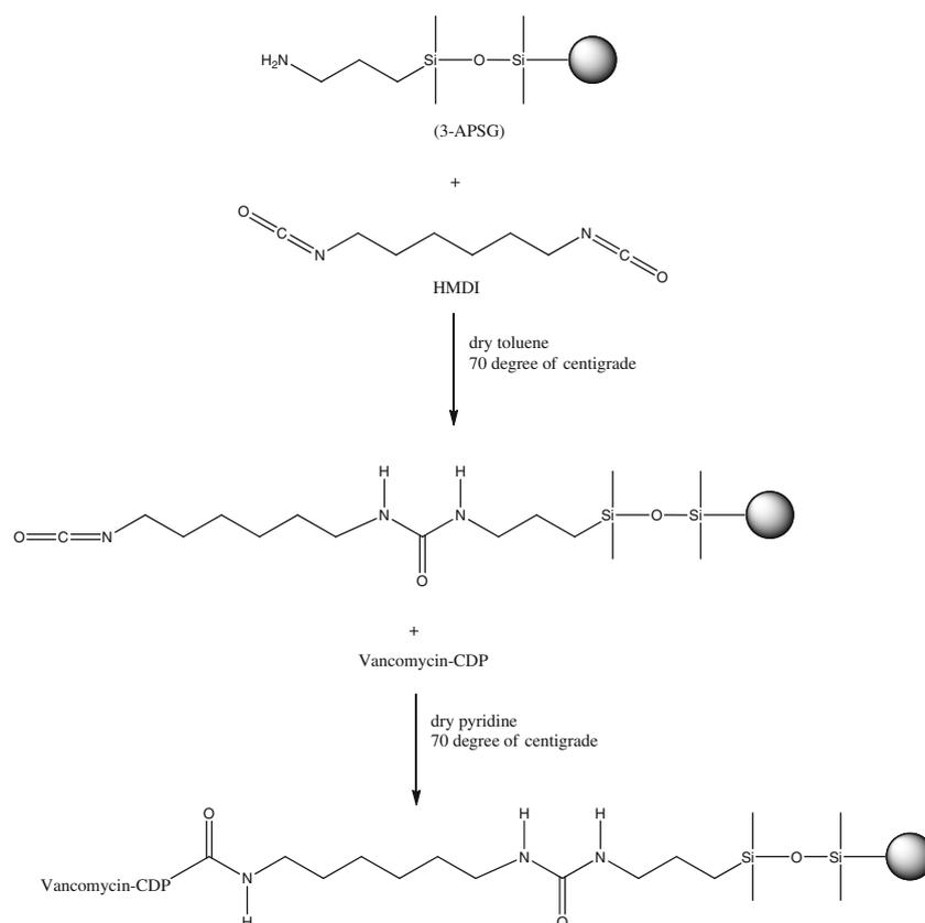
**Fig. 3.** Schematic diagram for preparation packing material of column B
