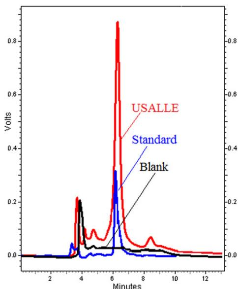
**Figure 3.** HPLC chromatograms of blank extract, direct injection of standard solution, and USALLE. Concentration of oleuropein in standard was 200  $\mu$ g/mL. Extraction conditions: pH, 4; organic phase, ACN/THF (50:50 v/v); organic phase volume, 2.5 mL; ultrasound time, 30 min; plant mass, 0.01 g; salt concentration, 25% w/v.
