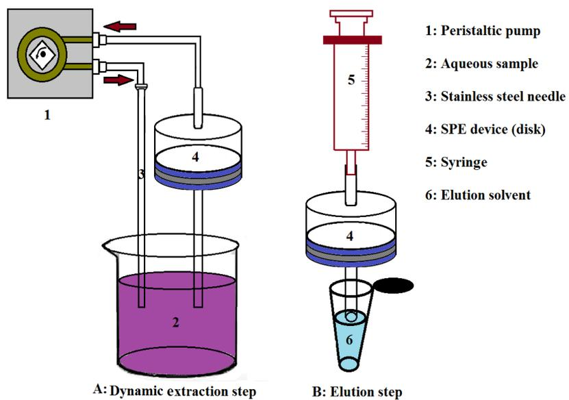
**Figure S-1.** The schematic of the SPDE-PTh/MWCNTs-disk procedure. A: dynamic extraction step, B: elution step.
