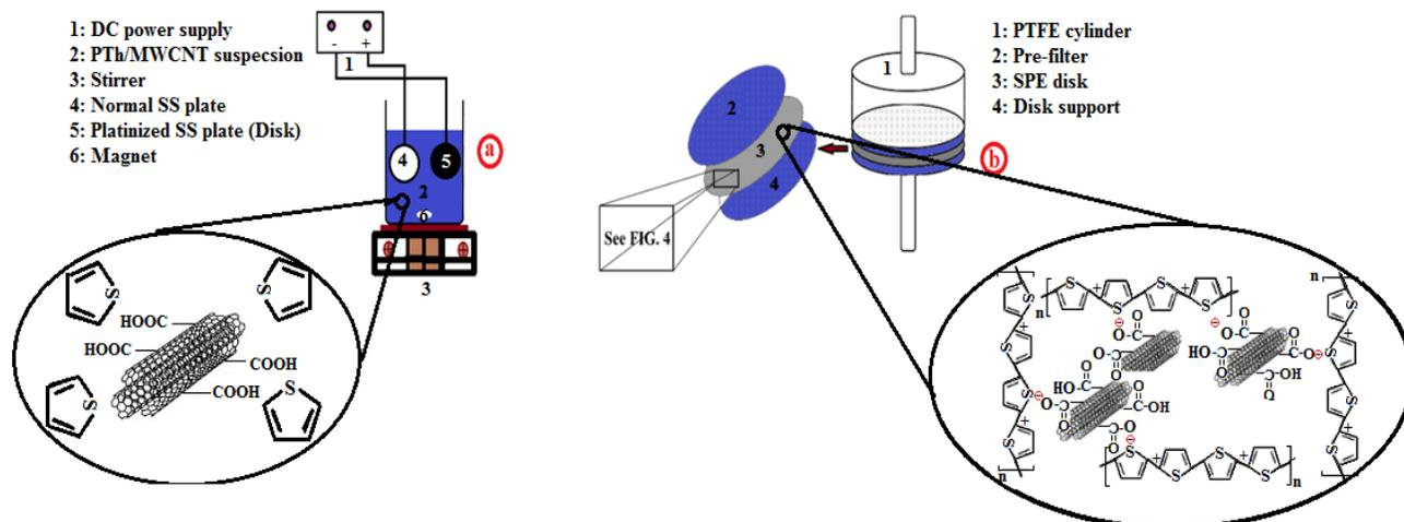
**Figure 1.** The Schematic of the Preparation of the SPE Disk Coated by PTh/MWCNTs Nanocomposite (a), Schematic of the SPE Column (b).
