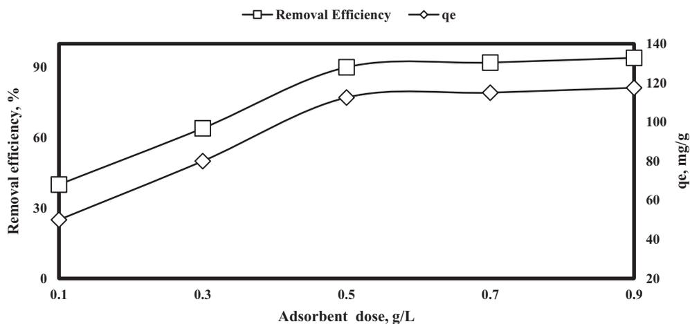
Figure 5. The effect of dose changes on Leaf-shaped ZIF-8 to MBD adsorption.
