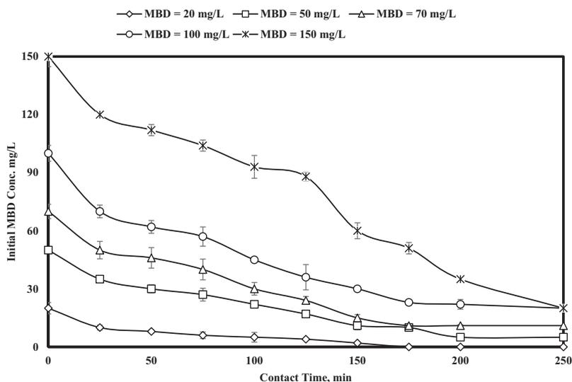
**Figure 4.** The effect of initial MBD concentration vs. contact time over MBD adsorption by Leaf-shaped ZIF-8 (pH = 9, adsorbent dosage = 0.4 g/L).
