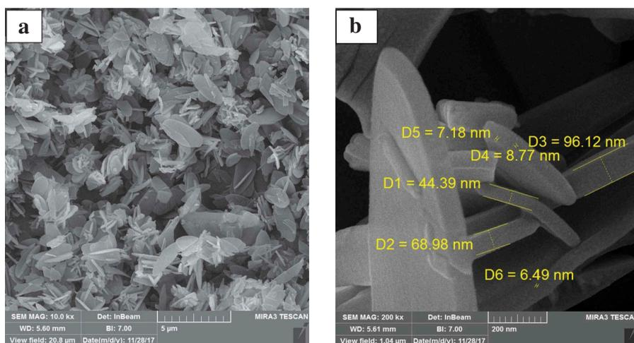
**Figure 2.** Field Emission-SEM image of prepared Leaf-shaped ZIF-8.
