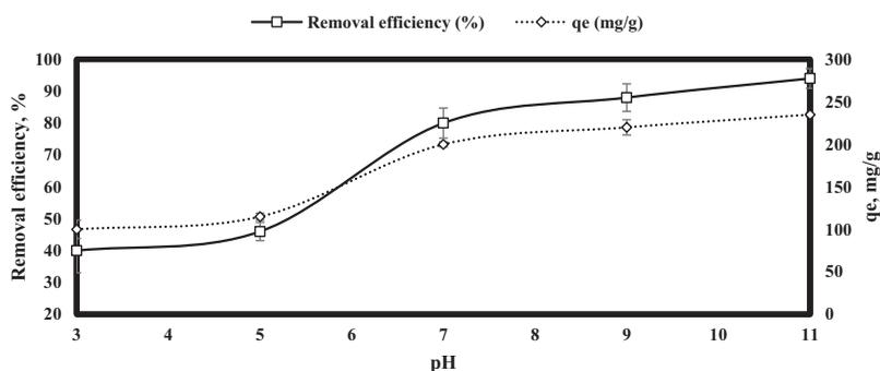
**Figure 3.** The effect of solution pH over MBD adsorption by Leaf-shaped ZIF-8 (Contact time = 30 min, initial MBD concentration = 50 mg/L, adsorbent dosage = 0.4 g/L).
