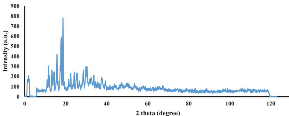
**Figure 1.** XRD pattern of prepared Leaf-shaped ZIF-8.
