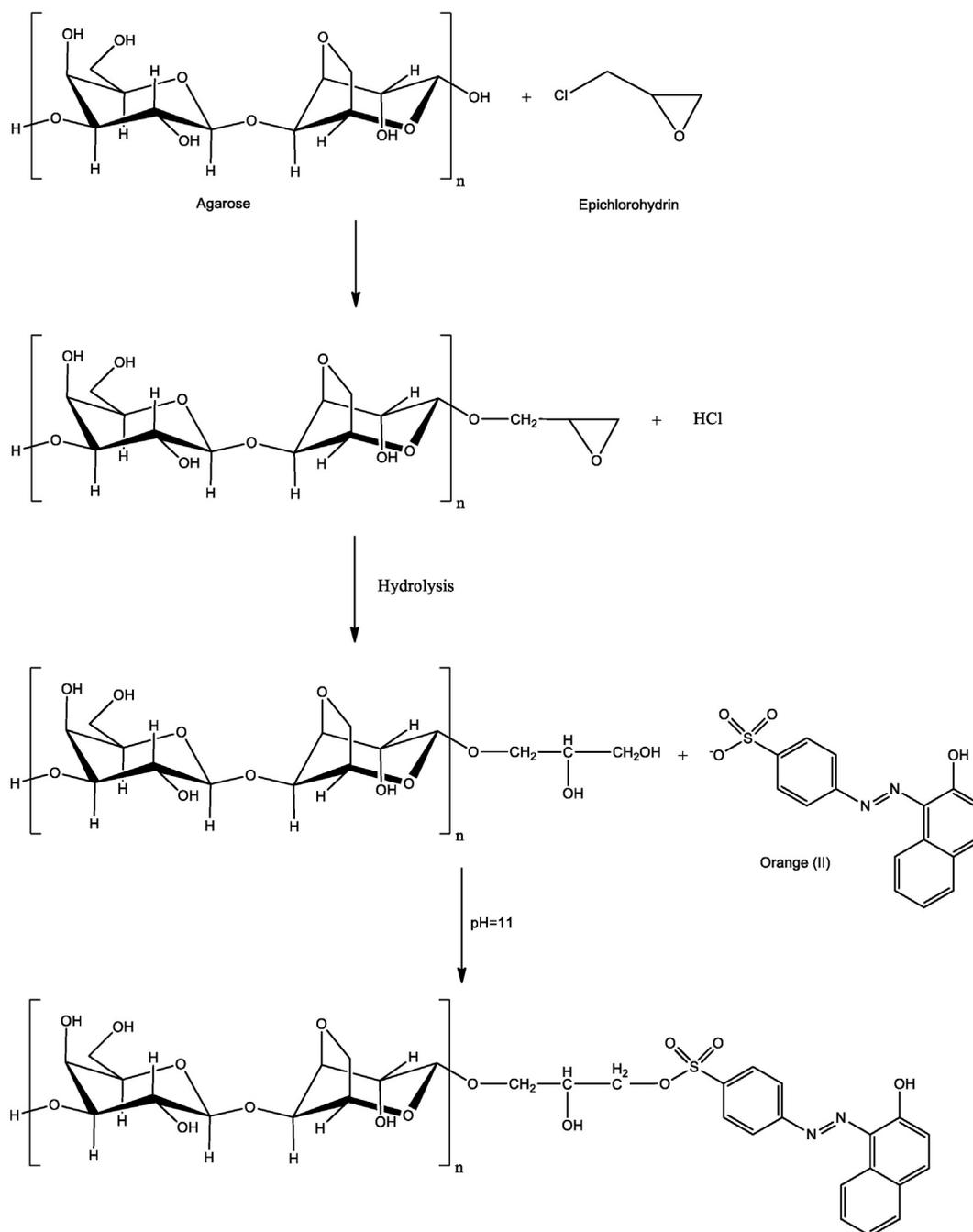
**Scheme 1.** The proposed mechanism of activation and dye bonding to agarose membrane.
