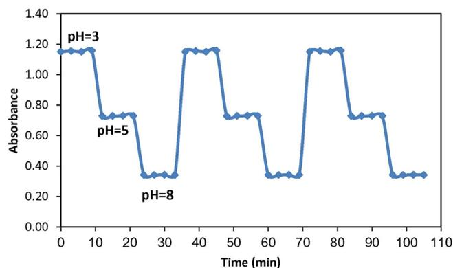
**Fig. 7.** Reversibility results of the optical sensor by changing the solution pH.
