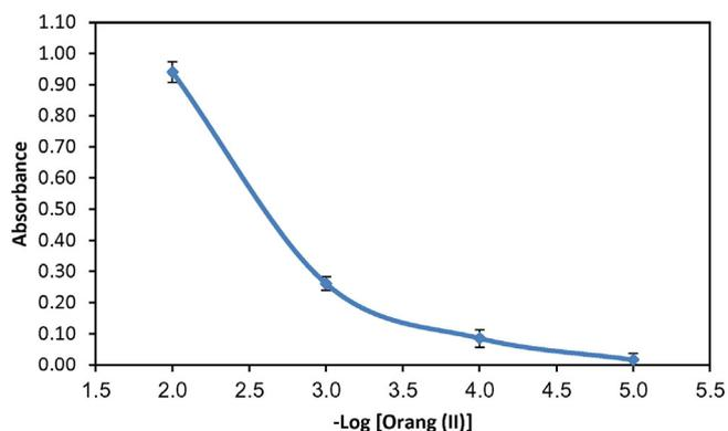
Fig. 3. Absorbance of the immobilized agarose membrane as a function of orange (II) concentration at 490 nm. Error bars are expressed as standard deviation.
