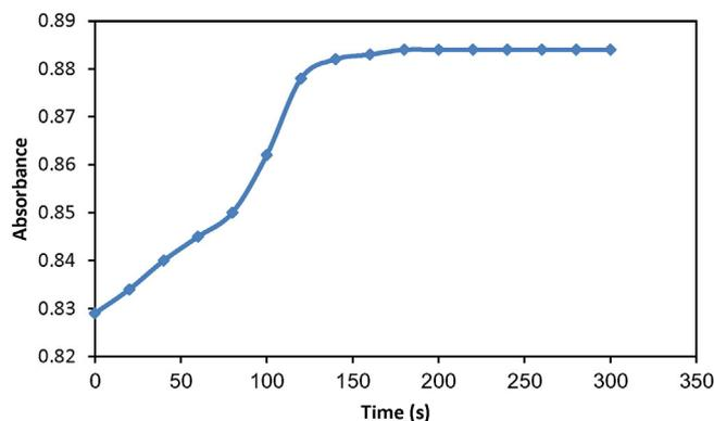
Fig. 5. Response time graph of the sensor as a function of time at 490 nm. Test conditions: sample pH, 4; immobilized orange (II) concentration,  $1 \times 10^{-2}$  mol L $^{-1}$ ; immobilization pH, 11.
