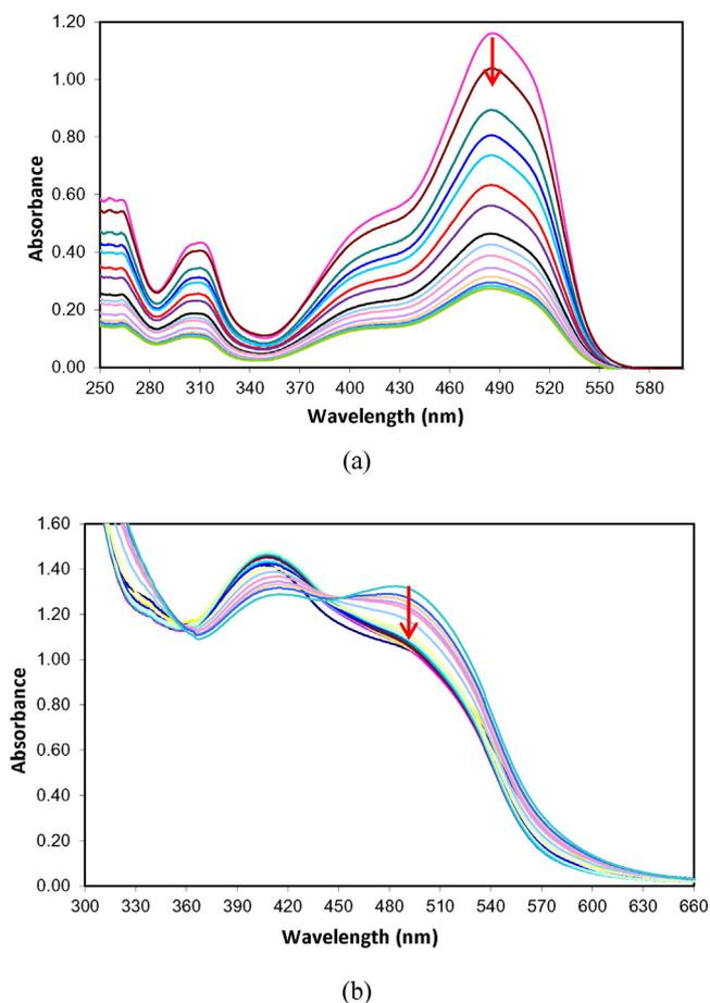
Fig. 4. Absorption spectra of immobilized orange (II) on agarose membrane (a) and orange (II) aqueous solution (b) at different pHs (3, 3.5, 4, 4.5, 5, 5.5, 6, 6.5, 7, 7.5, 8, 8.5, 9, 9.5 and 10). Concentration of orange (II) in aqueous solution was  $10^{-3}$  mol L $^{-1}$ .
