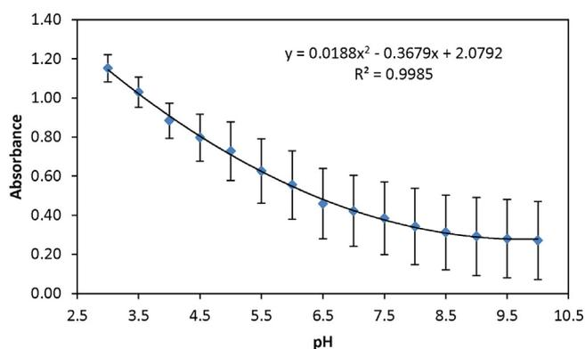
**Fig. 6.** Calibration curve of the optical sensor at 490 nm. Error bars are expressed as percentage of relative standard deviation.
