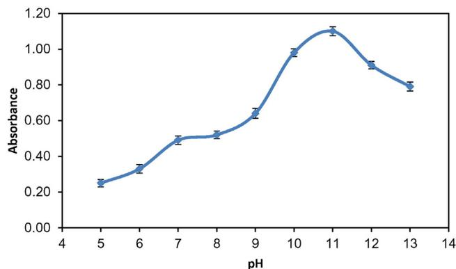
Fig. 2. Absorbance of the optical sensor as a function of the immobilization pH at 490 nm. The dye concentrations, 10<sup>-2</sup> mol L<sup>-1</sup>. Error bars are expressed as standard deviation.
