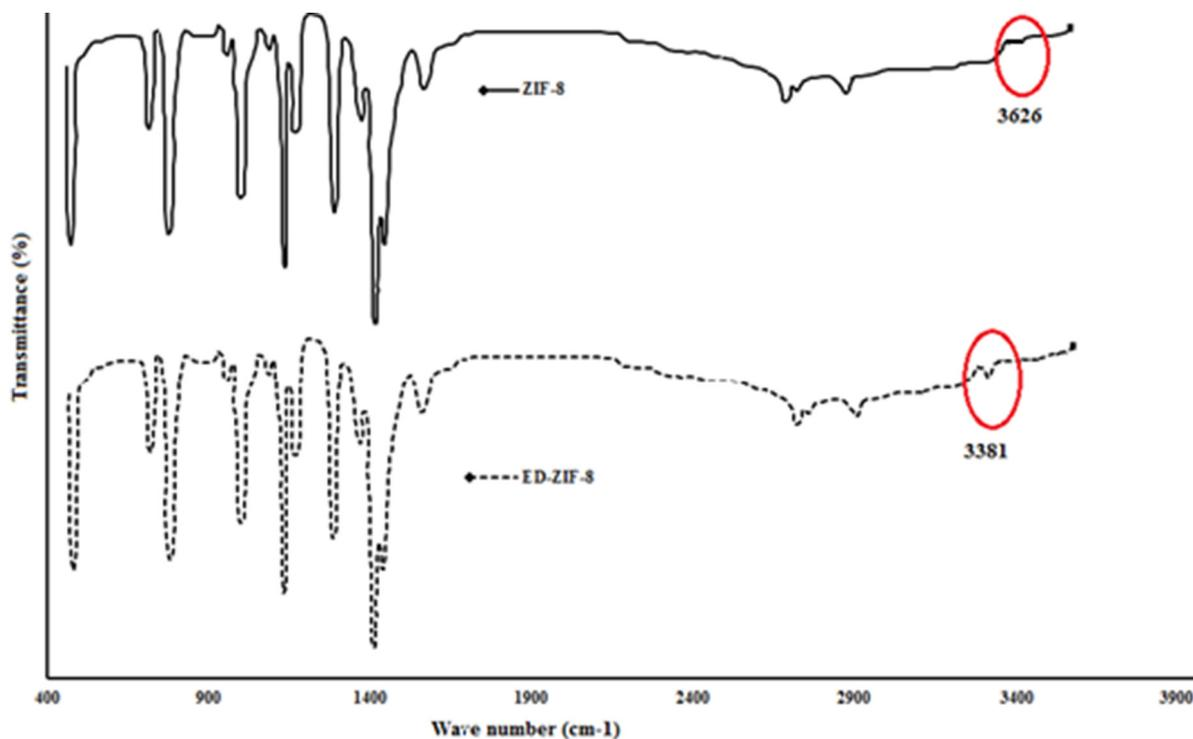
Fig. 3. FT-IR spectra of ZIF-8 and ED-ZIF-8.
