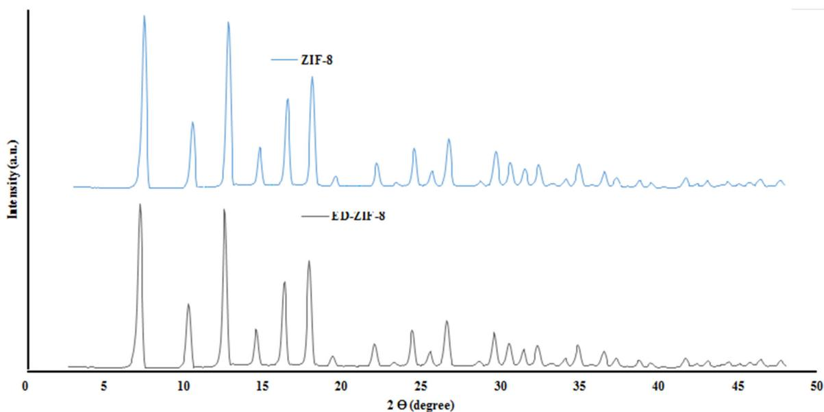
Fig. 1. XRD spectra of as-synthesis of ZIF-8 and Ed-ZIF-8.
