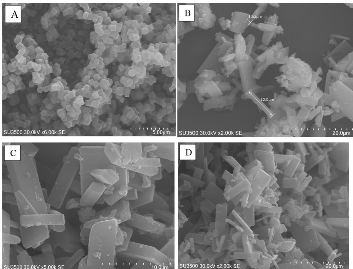
Fig. 2. FE-SEM image of ZIF-8 and ED-ZIF-8.
